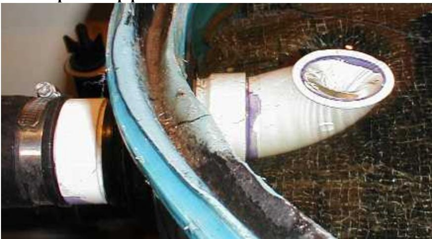
29. Inside the filter, connect a 90 degree elbow to the bulkhead fitting. As water enters this elbow to leave the filter it will create a whirlpool which will draw air down with the water. This will supply air with the water in the same manner that a venturi fitting would.
